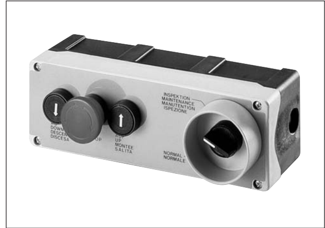
SC6-10 Flush protected pushbuttons with arrows + red mushroom with rotary release – STOP + Selector switch Two position 60° maintained with protection + yellow plate with wording in three languages In accordance with EN81
