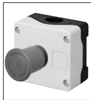
SC1-120 Red 'turn to release' mushroom button Ø 40 – STOP, With safety snap locking according to EN418 Black base and yellow cover
