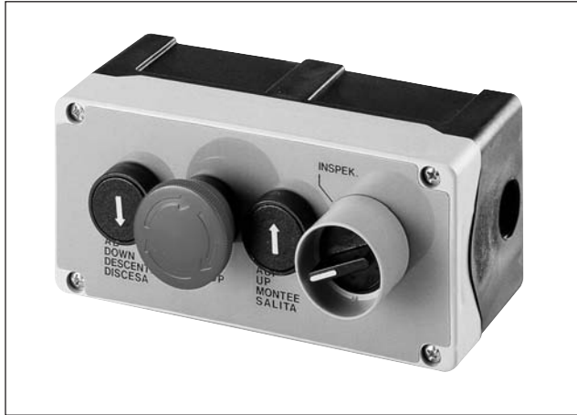
SC4-10 Two flush protected pushbuttons with arrows + red mushroom with rotary release – STOP + Selector switch Two position 60° maintained with protection + yellow plate with wording in three languages In accordance with EN81
